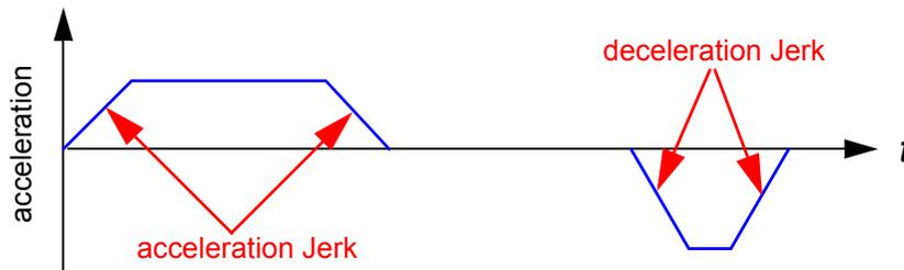
Fig 2. Acceleration profile with **smaller** value of jerk.
