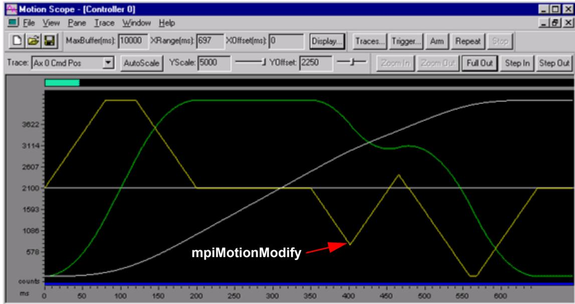
**New Firmware:** Notice that the acceleration changes less abruptly and that the velocity profile is much smoother.
