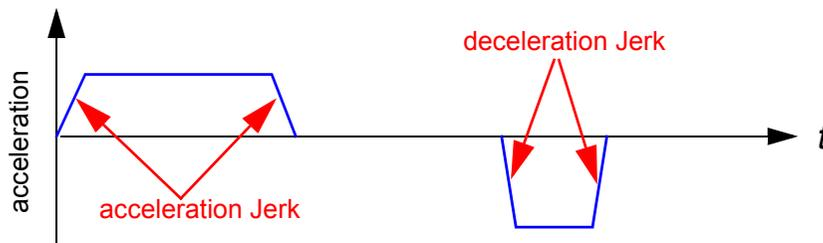
Fig 1. Acceleration profile with **larger** value of jerk.
