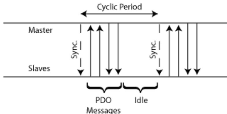
The advantage of this scheme is that it generates a predictable loading of data on the bus. The latency on transmitted data is predictable, but the latency is not the absolute minimum that can be achieved.
