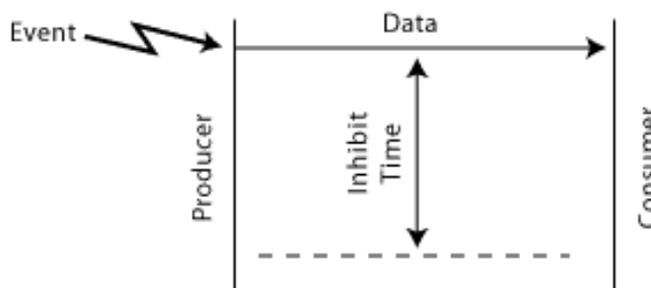
The advantage of this type of messaging is that short reaction times are attainable, but this is accomplished at the expense of variable network traffic, and the possibility of saturating the network. In many cases, the reaction time is not significant in relation to other time delays in the system (ex: the user's application or delays in task switching).
