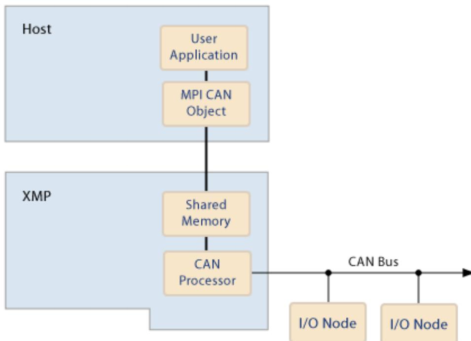
The XMP operates as a master node on the network with all the IO nodes being slaves. This arrangement implies that there may only be one XMP on any CAN Network.
