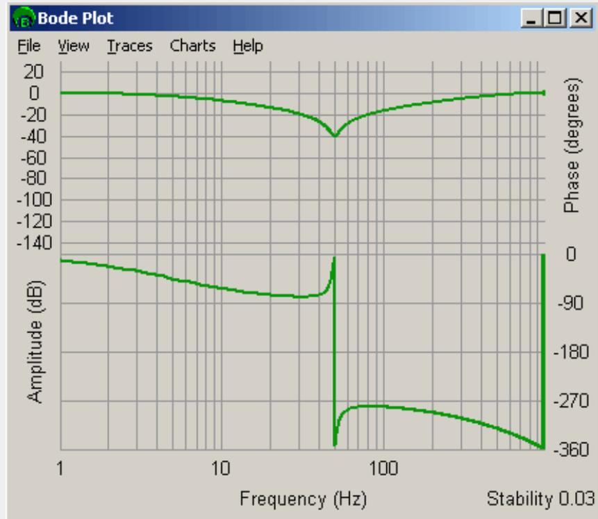
Example of a 50 Hz center / 50 Hz Bandwidth / -40 dB Gain Resonator filter. Note that phase wrapping gives the illusion that the phase drops 360 degrees after the center frequency.
