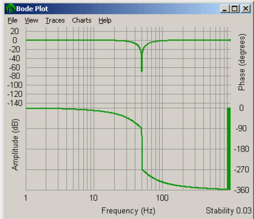
Example of a 50 Hz Center / 50 Hz Bandwidth Notch filter. Note that phase wrapping gives the illusion that phase drops 180 degrees after the center frequency. The phase raises by 180 degrees.
