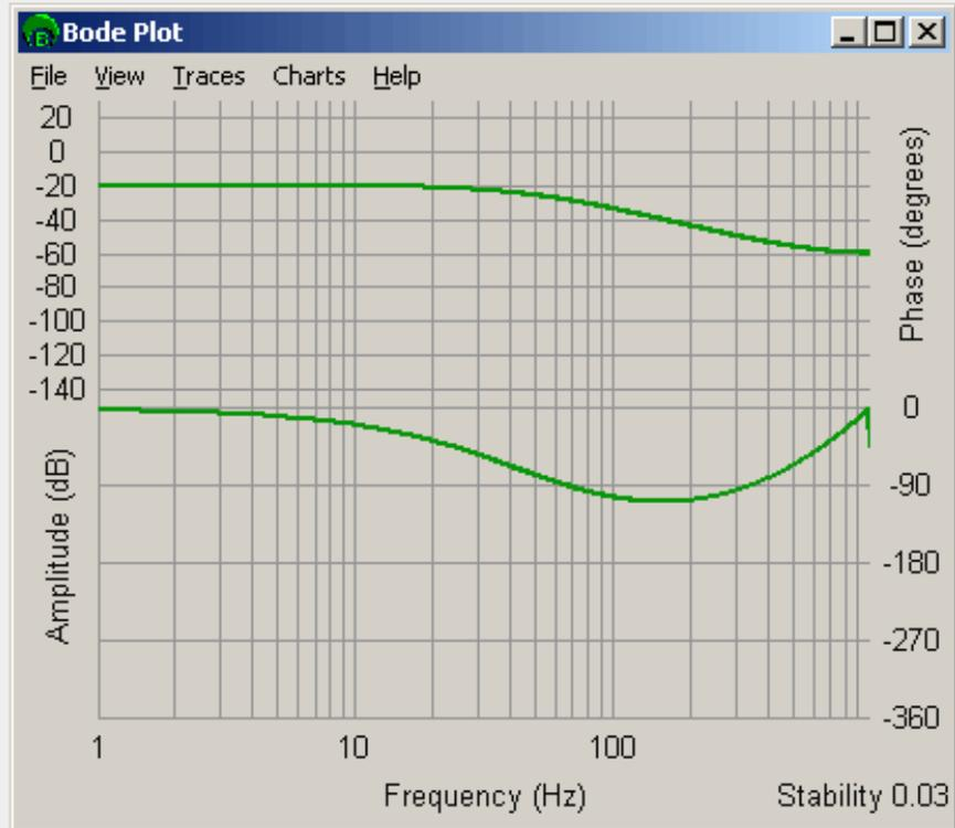
Example of a -20 dB low frequency gain / -60 dB high frequency gain / 50 Hz center lead lag filter.
