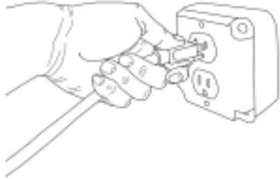
**1** Shut down your computer and follow the manufacturer's instruction for opening the computer and installing hardware. You should be properly grounded and avoid touching the gold contacts on the XMP/PCI controller.
