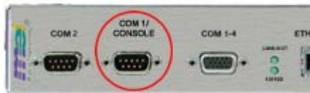
The short between these two pins indicates the presence of a valid console device and is detected during system initialization by the eXMP, thereby enabling the Console output to COM1. This can be done with either an inline adapter or modifications to the Null Modem cable itself.
