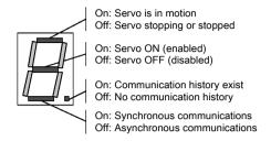
Only the Servo OFF light segment will light up before connecting to the network after turning on the power supply.
