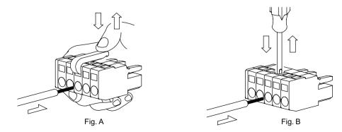
3. Insert the wire core into the opening and then close the opening by releasing the lever or removing the screwdriver.
