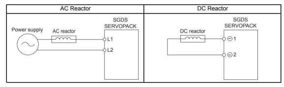
Note: 1. The DC reactor's  $\ominus$  1 and  $\ominus$  2 terminals are short-circuited before shipment. Remove the lead wire between these two terminals and connect the DC reactor.
