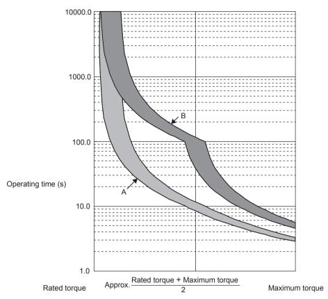
Note: The overload protection characteristics of A and B in the figure are applicable when the SERVOPACK is combined with one of the following servomotors.
