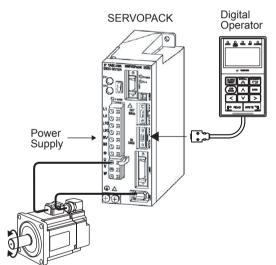
The motor can be operated using only the digital operator. This makes it possible to check the servomotor rotation direction and set the speed during machine setup and trial operation without connecting the host controller.
