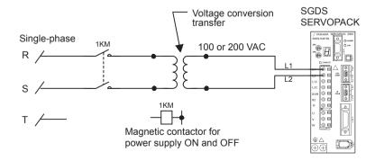
Fig. 5.1 Single-phase Power Supply Connection Example
