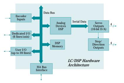
High-Performance DSP Architecture The LC/DSP uses a high-performance DSP to execute real-time motion control algorithms, offloading non-real-time functions to the host. The LC/DSP buffers commands from the host and stores motion and I/O sequences on-board.
